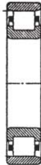
Cylindrical Roller Bearing without adapter sleeve.
